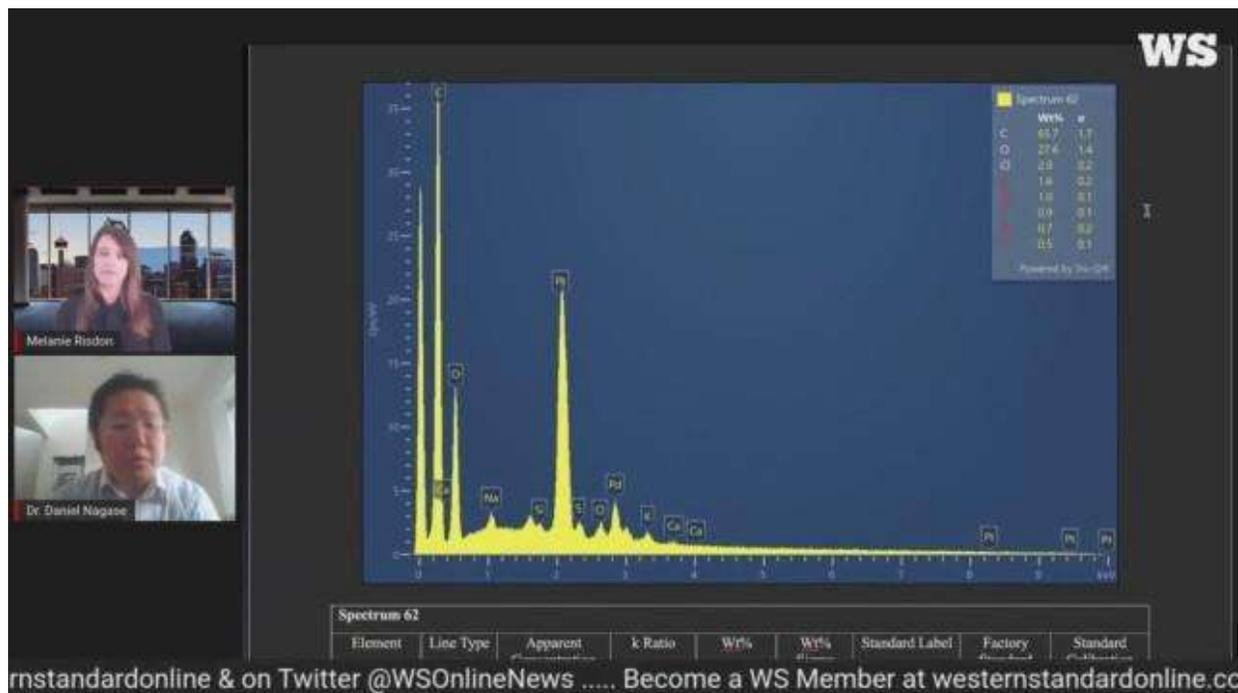
Same story again. Carbon, oxygen, some silicon, some sulphur, some potassium this time, a bit of calcium. But no nitrogen, no phosphorus. So, nothing we saw in that photo was of biological origin. It appears to be a primarily carbon-oxygen structure. So
