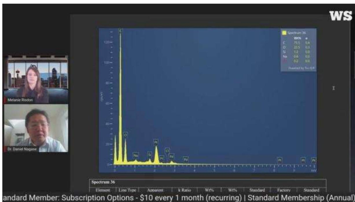
So, if this was a salt crystal, we'd expect to see sodium and chloride. And what do we see in square 36? It's carbon, oxygen, a little bit of sodium, and a little bit of chloride. But again, it's carbon, oxygen, platinum, which was an artefact because we added that to the sample, and a little bit of silicon. That's really unusual. And let's scroll down to spectrum 37.
