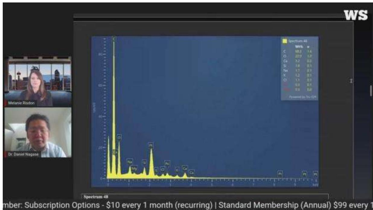
So, this spectrum 48 didn't have any thulium, it's just carbon, oxygen, magnesium, silicon, and a bit of sodium and calcium. And let's keep scrolling down.
