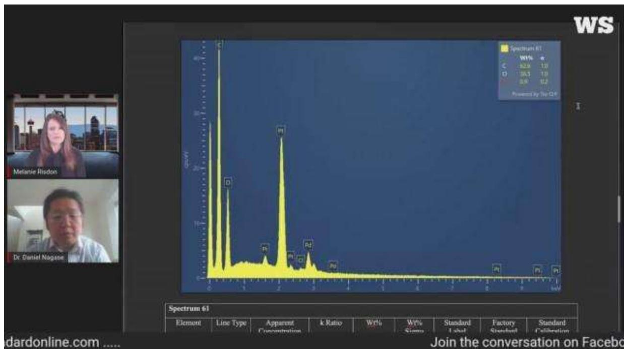
So, again, pretty similar story. Carbon, oxygen. For some reason, the square under spectrum 61 accumulated a lot of platinum. But again, platinum could be something that we added to the sample just to protect the sample from being burnt up in the first second or two of exposure to an electron beam. But again, no signs of nitrogen or phosphorus. It's just carbon and oxygen. So, we know that there was nothing biological in spectrum 61 in that square. And then spectrum 62,
